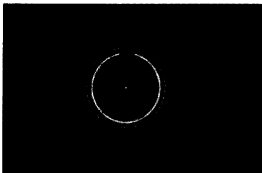
FIG. 2. Electron diffraction pattern of platinum in a reduced catalyst.
